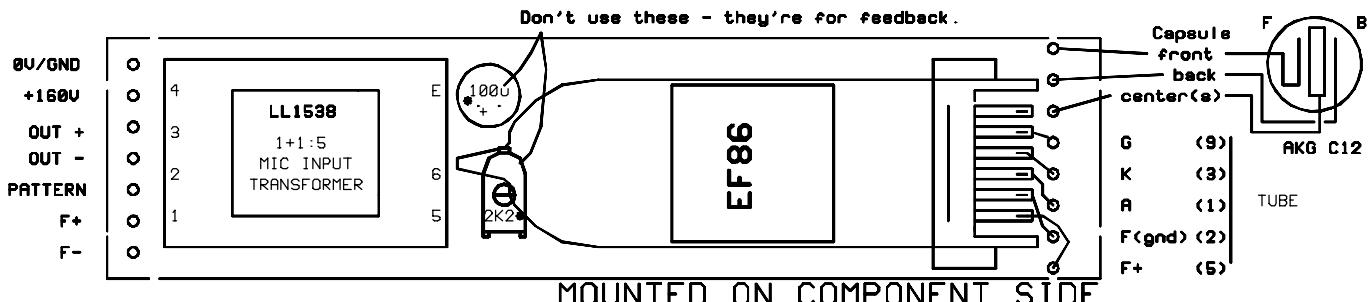
MOUNTED ON COMPONENT SIDE
